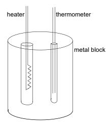
The voltage, V, applied to the heater and the current, I, through it are measured. The temperature rise is related to the other quantities by the following equation, providing no heat is lost to the surroundings.
