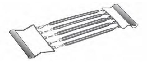
An expander consists of 5 springs in parallel held between two handles.
