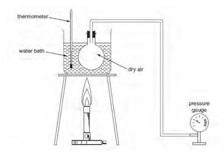
The change of pressure was noted as the temperature was increased. The results are shown on the graph below.
